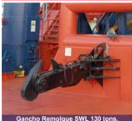
Gancho Remolque SWL 130 tons.
